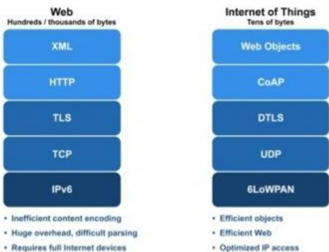
Figure 2. Comparison of Web and IoT protocol stacks
